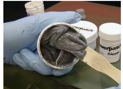
Mix 2-part paste sealant to a uniform grey color
