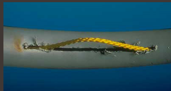
Rope burn-through at a bend
