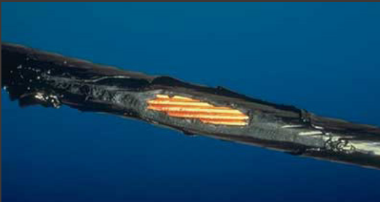
Jacket burn-through due to excessive sidewall pressure
