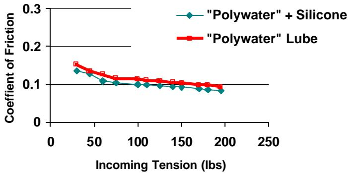
**Figure 2. Effective Coefficient of Friction With "Polywater®" Lubed Cable versus "Polywater® Plus Silicone" Lubed Cable**
