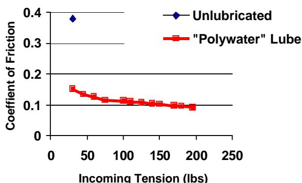
Figure 1. Effective Coefficient of Friction With "Polywater®" Lubed Cable versus Unlubed Cable
