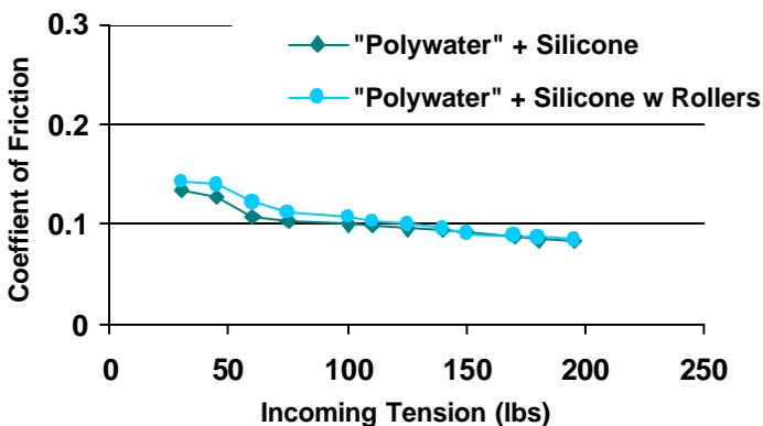
**Figure 3. Effective Coefficient of Friction With "Polywater® Plus Silicone" Lubed Cable versus "Polywater® Plus Silicone (with Mini-Rollers)" Lubed Cable**
